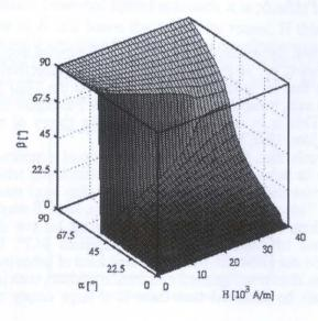
Figure 7. The angle between the flux density vector in the {110} plane and the (001) axis as a function of the magnitude and the direction of the applied field
