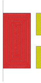
Fig. 2. Transient academic example ( Multi Coil Model ): magnetizing coils (green) and conductive sample (red).
