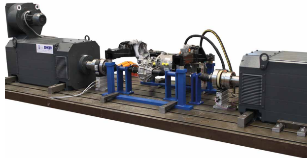
Figure 6: Test bench at the Institute of Electrical Machines (IEM) for drive train of electrical vehicle. Two load machines. Subframe of the vehicle with sub-construction for test bench: Electrical machine, gear and differential, fixed with three bearings in the subframe. Side shaft and wheel bearing with adaption to load machines on each side. Water cooling system for electrical machine and converter.
