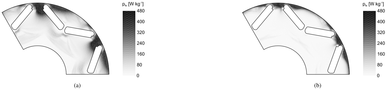
Fig. 6. Iron-loss distribution inside the rotor at 18000 \text{ min}^{-1} and 25 \text{ Nm} for (a) q = 1, w = \tau_p and (b) q = 2, w = \tau_p .
