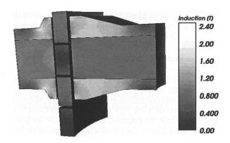
can be obtained from FE simulations. In this way the flux coupling in the coils can be determined in every position (x) of the coil assembly. The flux density at each coil ( $B_n$ ) can be put into relation of the flux density of all coils according to equation (2) and is referred to as the axial position dependent current factor ( $k_{I,n}(x)$ ):
