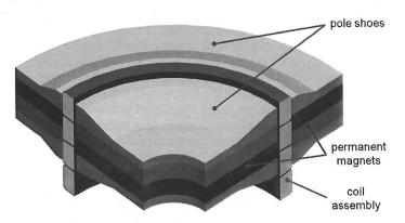
**Figure 3.** CAD drawing of the drive
