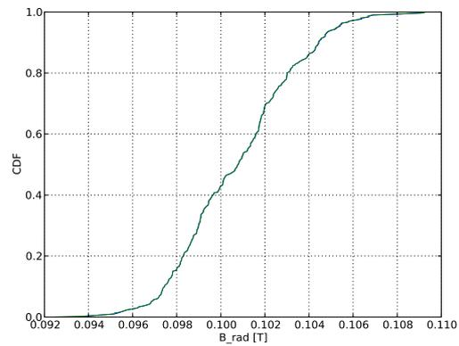
Fig. 5: Cumulative distribution function (CDF) of the flux-density at the evaluation point at the magnet's middle (angle  $0^\circ$ ).
