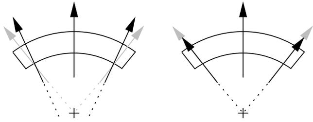
(a) Error type A: deviation of radial magnetization towards unidirectional magnetization. (b) Error type B: deviation of local magnetization strength, weakening towards the magnet edge.
