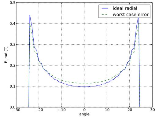
Fig. 4: Comparison of the radial flux-density along the chosen evaluation line for ideal flux density and worst case flux density (dashed).
