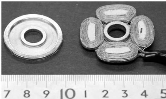
Fig.1. Active hybrid magnetic bearing components; rotor with bias PM (Left) and 4 pole stator (right).
