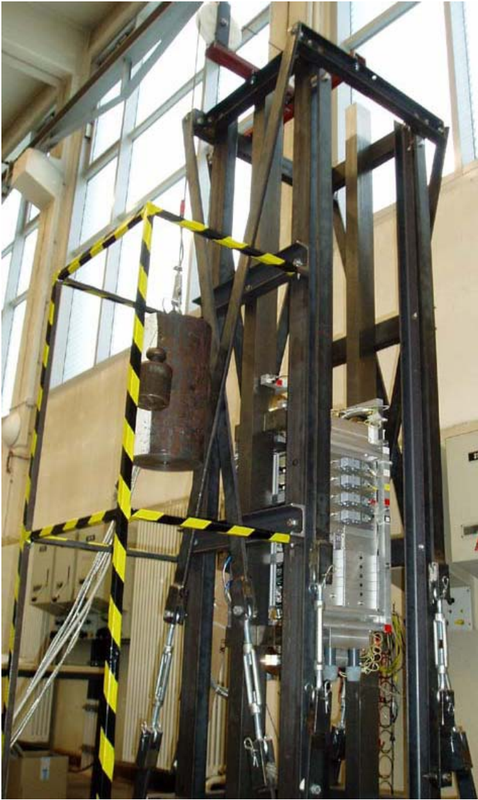
Figure 2. Electromagnetically guided elevator test bench.
