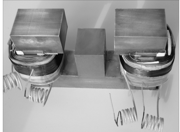
Figure 1: Omega actuator without permanent magnets [3].
