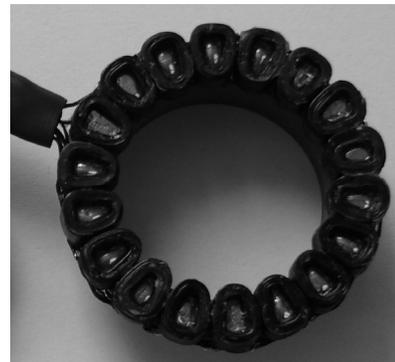
Fig. 6: Stator with winding of the drive prototype.
