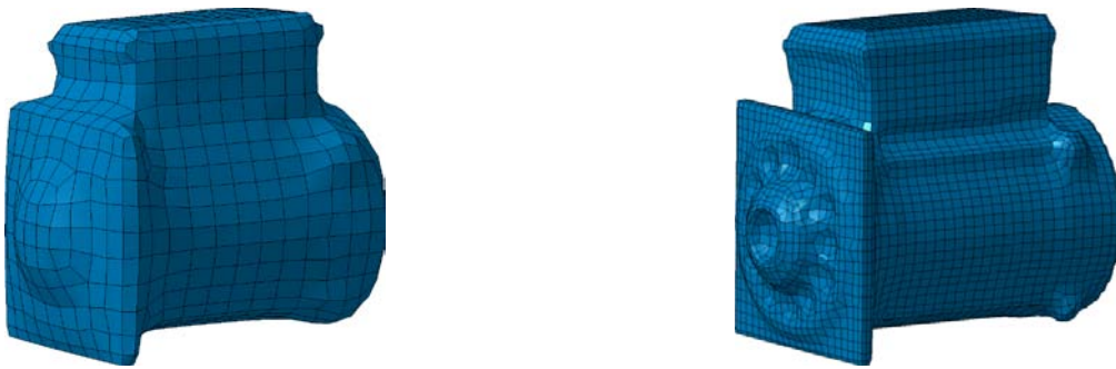
Figure 4 Acoustic meshes for different maximum simulation frequencies (left: 2 kHz, right: 5 kHz)
