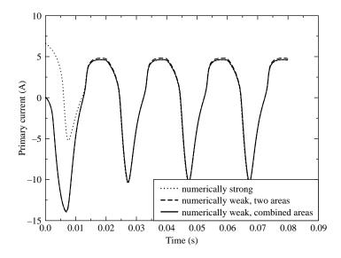
Figure 8. Comparison of numerically strong- and weak-coupled simulation for  $R=5\,\Omega$
