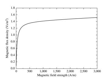
Figure 2. Material characteristic of M250-35 A magnetic steel
