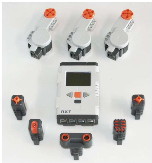
Fig. 1. LEGO Mindstorms NXT hardware of the standard education kit: five sensors (light, sound, ultrasonic, and two touch sensors), three servo motors, and programmable NXT brick.
