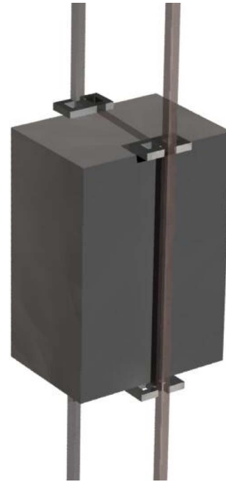
Fig. 5. Elevator car guided by four TAAAs.
