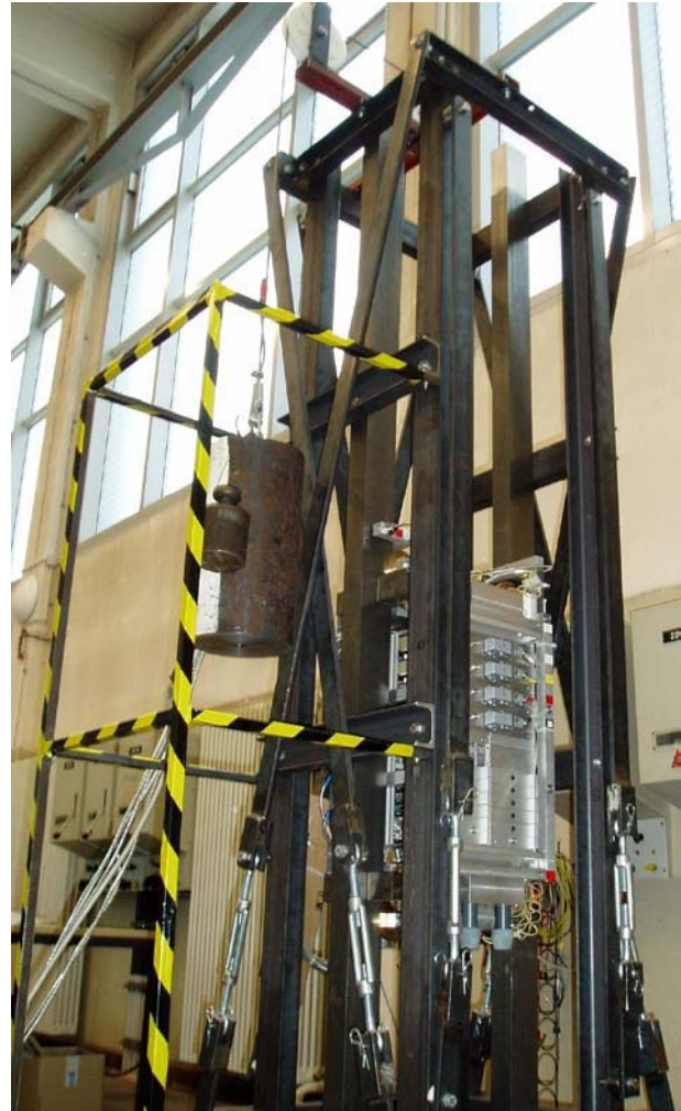
Figure 1: Electromagnetically guided elevator test bench.
