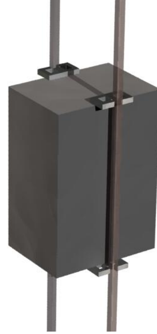
Fig. 4. Elevator car guided by four TAAs.
