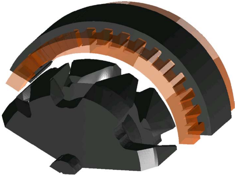
Figure 1. Rotor and stator (with windings) of a CPA
