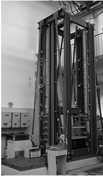
Figure 2: Ropeless elevator test bench.
