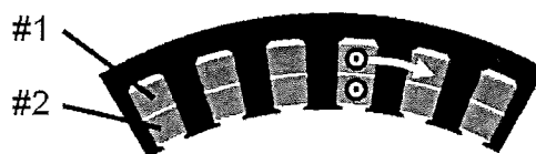
Fig. 2: Two-layer winding (with displacement).
