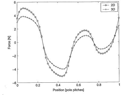
Figure 13. Comparison of the forces computed with the 2D and 3D models; xp ranges from 0 to 1, mean of the  $\underline{b}$  and  $\underline{h}$  formulations,  $I=200~\mathrm{A}$
