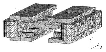
Figure 1. Geometry of the linear actuator
