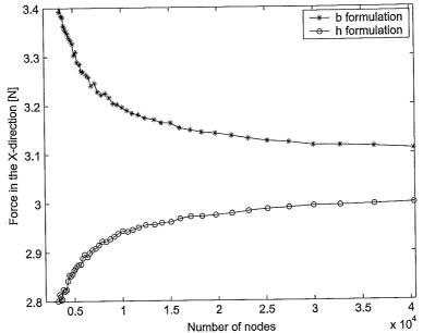
Figure 9. Convergence of  $F_x$  computed with the eggshell method; 2D model,  $\underline{b}$  and  $\underline{h}$  formulations,  $x\underline{p}=0.125$  pole pitches, I=0
