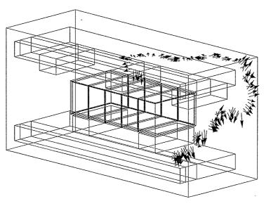
Figure 5. Vector potential a on the boundary, such that its line integral on  $\partial \Gamma_{h1}$  equals  $\varphi_b$  and  $\operatorname{curl}(a).n = 0$  on  $\Gamma_b$
