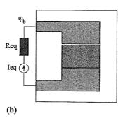
Figure 2. Coil modelling (a) explicit definition in the geometry; and (b) equivalent magnetic circuit
