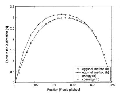
Figure 10. Comparison of the force computed by the eggshell method and the differentiation of the energy and coenergy; 2D model, xp ranges from 0 to 0.5 pole pitches, I=0
