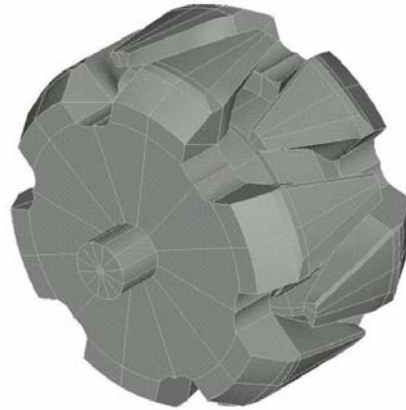
Fig. 4: Rotor with claws (iron part).
