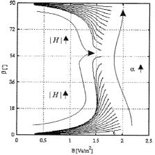
Figure 9. Lines of constant  $\alpha$  in the  $\vec{B} - \beta$  plane, with parameter  $|\vec{H}|$
