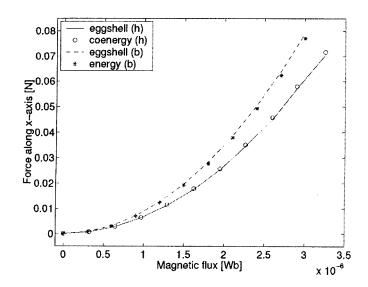
different formulations when evaluating the Maxwell stress tensor, i.e. for instance, not to mix the  ${\bf h}$  field from a  ${\bf h}$ -formulations with the  ${\bf b}$  field from a  ${\bf b}$ -formulations, although this may seem a good idea from the point of view of the individual accuracy of the different fields. Figure 4 shows indeed that the forces computed with the mixed expression
