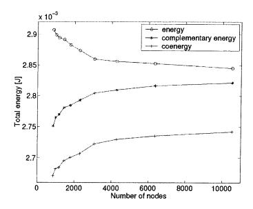
Figure 2. Energy Ψ, coenergy Φ and complementary energy  $\int_{\Omega} \mathbf{b} \cdot \mathbf{h} \, d\Omega - \Phi$  as a function of the number of nodes. The difference between energy and complementary energy is a measure of the global discretisation error
