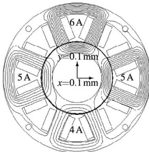
**Figure 2.** The geometry and field distribution of the discussed radial AMBs
