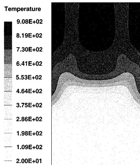
Fig. 4. Temperature distribution caused by the heat source distribution of Fig. 3 in degrees C.
