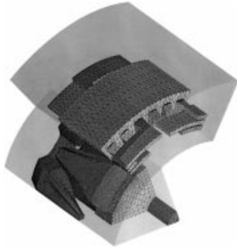
Fig. 1. Discretized FE model with translucent air regions.
