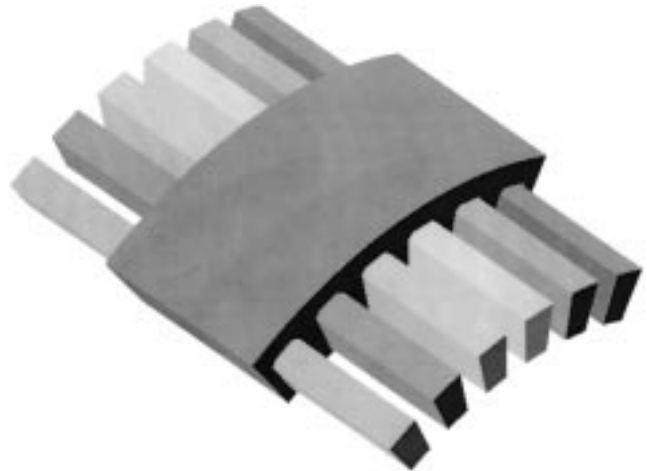
Fig. 2. Simplified winding region.
