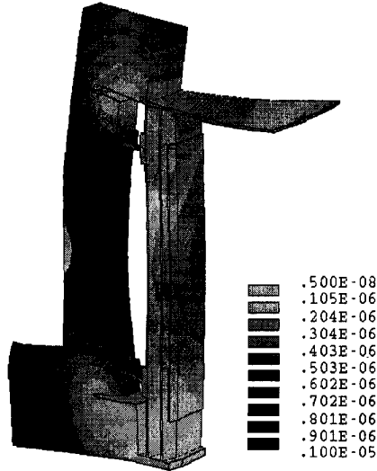
Fig. 4. Real part of the deformation of the furnace (m)
