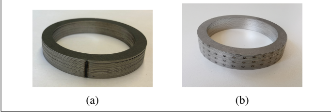
Figure 3: (a) Line-weld sample and (b) Spot-weld sample.
