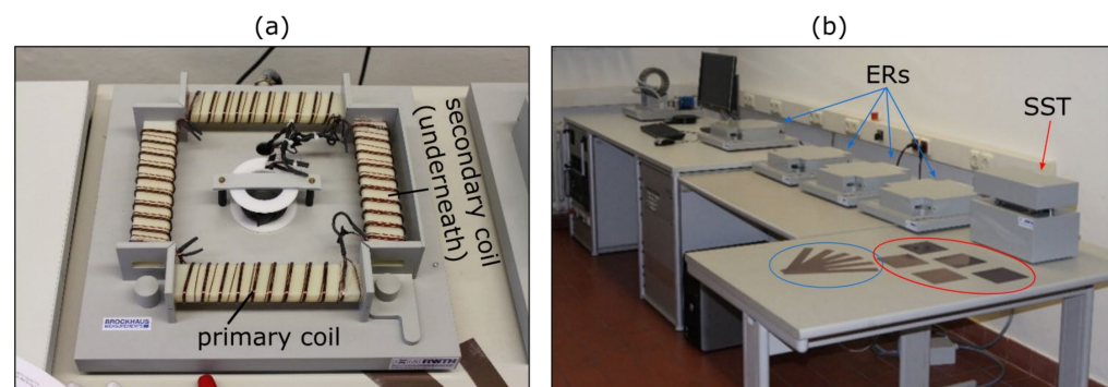
Figure 5. (a) Epstein frame (ER) with primary and secondary coils around the four limbs, (b) lab with four ERs and one single-sheet tester (SST) as well as several ER strip samples (blue circle) and several rectangular SST samples (red circle).
