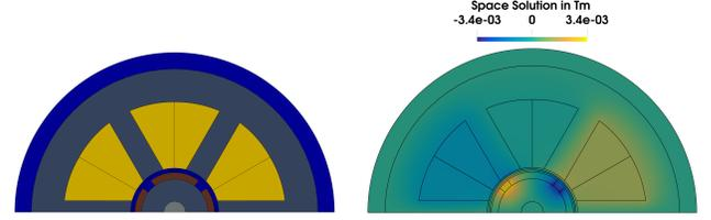
(a) Geometry of the synchronous machine including a non-conformal airgap
