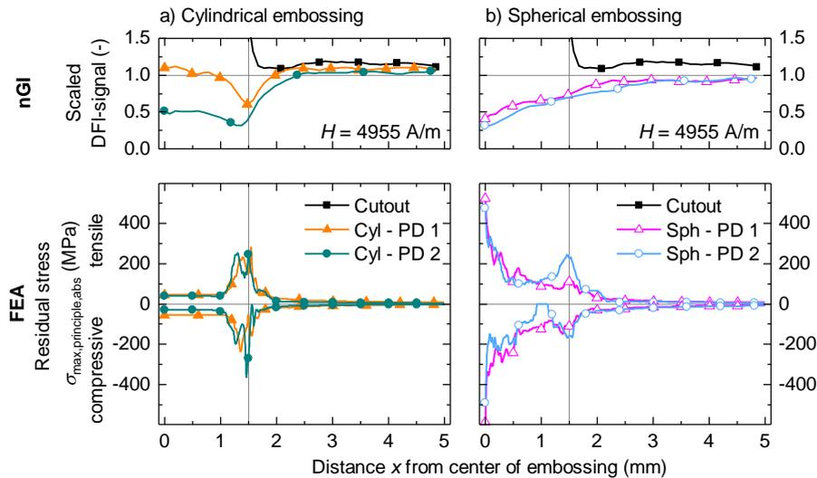
Fig. 9 Comparison of scaled DFI-signal at a magnetic field strength  $H$  of 4955 A/m and numerically analyzed residual stress distributions  $\sigma_{max,principle,abs}$  of a), cylindrical, and b), spherical embossings.
