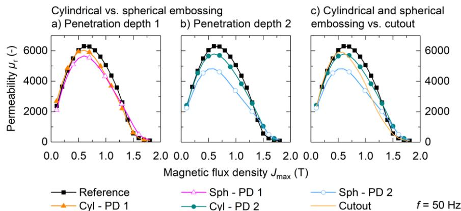
Fig. 8 Magnetic permeability  $\mu_r$  of cylindrically and spherically embossed specimen fabricated with a), penetration depth 1, and b), with penetration depth 2, compared to reference material and c), comparison of reference material, cylindrically embossed specimen with a penetration depth of 240  $\mu\text{m}$ , spherically embossed specimen with a penetration depth of 230  $\mu\text{m}$  and flux barrier manufactured as cutout.
