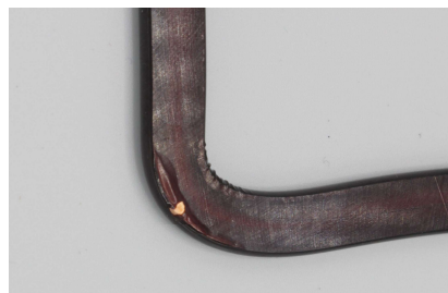
Fig. 13: Close-up of a defect in the surface insulation.
