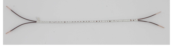
Fig. 4: Specimen for PDIV measurement of enameled rectangular wires [8].
