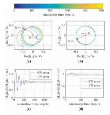
Figure 4. Rotor flux loci vector and error in amplitude of rotor flux linkage vector in dependency of simulation time step *ts* for the operating point  $\hat{f}_1 = 5 \text{ A/mm}^2$ ,  $f_2 = 5 \text{ Hz}$  with zero flux starting condition (SOA) and with analytical starting condition (*nonlinear hybrid*)
