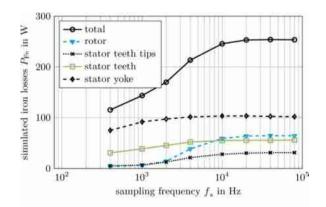
**Figure 3.** Dependency of the simulated iron losses on the sampling frequency  $f_s$  of the transient FEA
