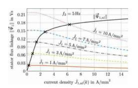
Figure 2. Interpolation of the stator flux linkage vectors to determine the no-load stator current density  $\hat{J}_{1,nl}$  by (5)
