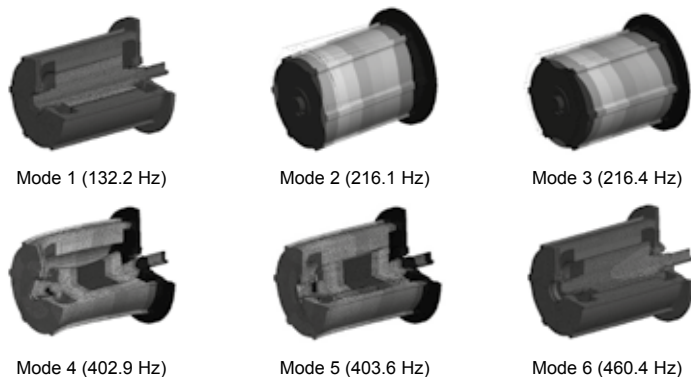
Figure 8: First six modes of the PMSM including mechanical structure.
