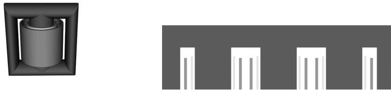
Fig. 2. Applied transformer models: a) single-phase transformer S = 100 MVA, b) three-phase transformer S = 120 MVA
