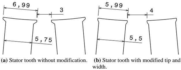
Fig. 5. Various stator tooth geometries of the original and modified motor.
