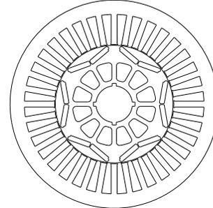
Fig. 3. Geometry of the initial motor.
