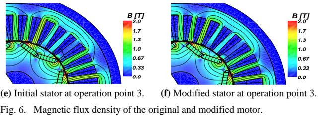
Fig. 6. Magnetic flux density of the original and modified motor.
