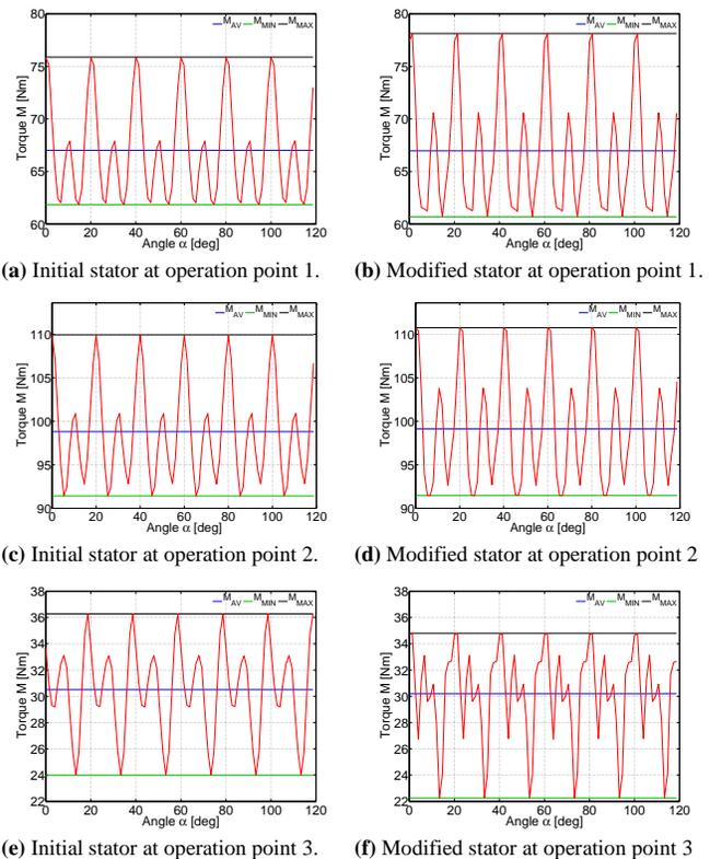
Fig. 7. Torque with the initial and modified motor geometry.
