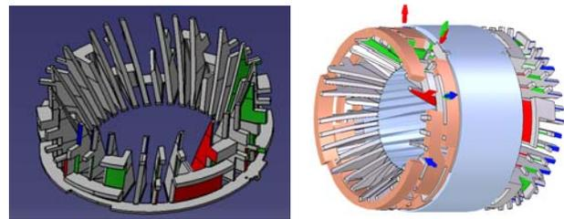
(a) Lamella structure of the end caps. (b) End caps and stator.
