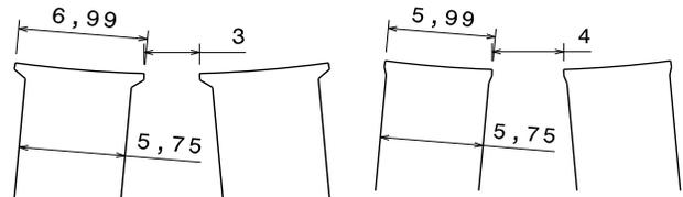
(a) Stator tooth without modification. (b) Stator tooth with modified tip.
