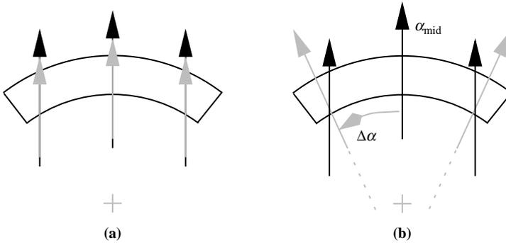
**Notes:** (a) Constant remanence flux-density weakening, modelled by parameter  $\xi_1$ ; (b) angle deviations, growing in dependence of their distance towards the magnets edges, modelled by parameter  $\xi_2$
