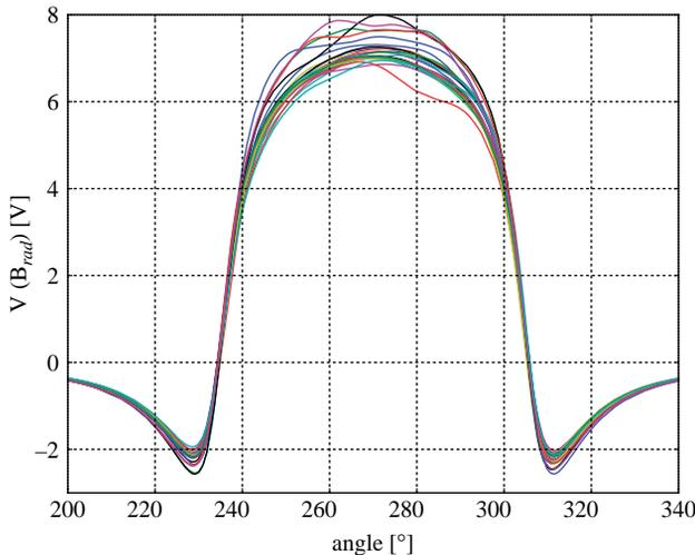
**Figure 4.** Plot of Hall-voltages of the radial flux-densities of 26 magnets measured 1.6 mm above each magnet's surface
