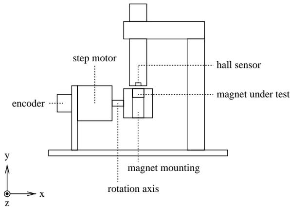
**Figure 3.** Sketch of the test-bench used for measuring the magnets' radial flux-density components
