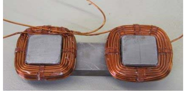
Fig. 4 U-shaped hybrid actuator without permanent magnets.
