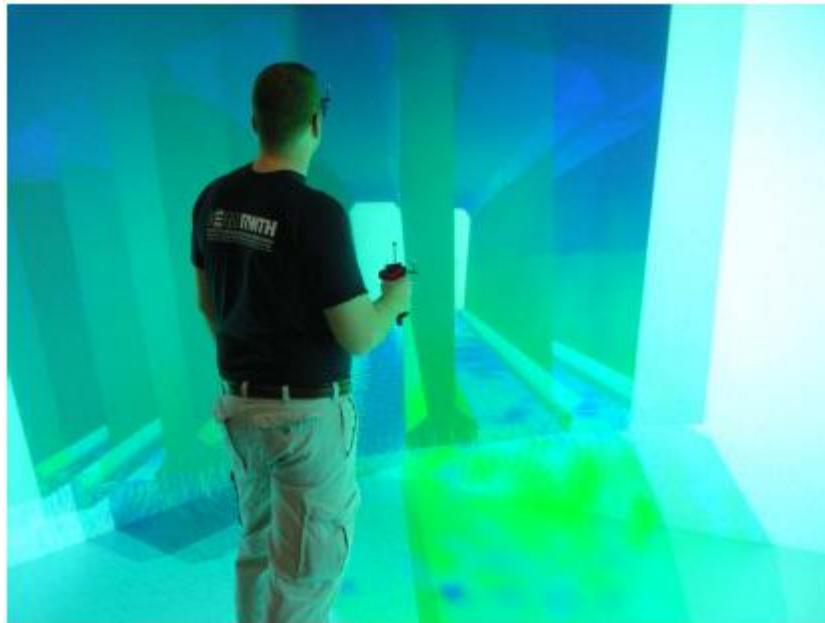
Fig. 2. Virtual reality (VR) environment. Electromechanical device presented in a VR-cave.
