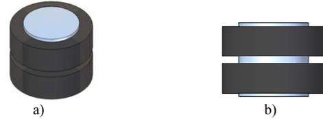
Fig. 3. Unskewed magnets on the linor surface of one pole pair: a) Dimetric view; b) Front view.
