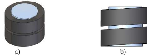
Fig. 5. Plane skewed magnets on the linor surface of one pole pair: a) Dimetric view; b) Front view.
