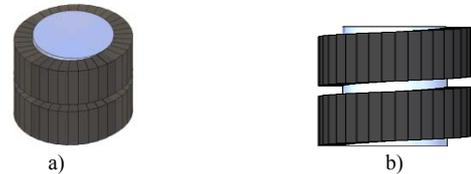
Fig. 4. Skewed magnets on the linor surface of one pole pair: a) Dimetric view; b) Front view.
