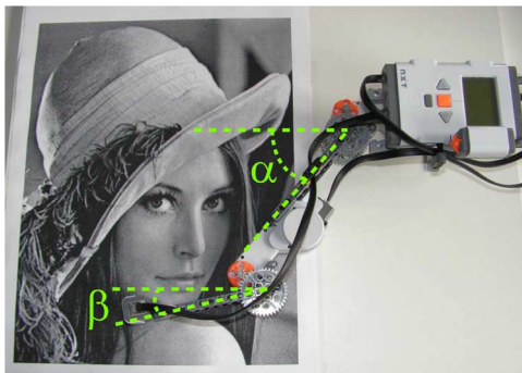
Fig. 11. The 2-D scanner scans a poster image using the NXT light sensor. The position of the sensor is determined by a two-joint robot arm controlled by servo motors. The angle position of the two joints can be described by the angles \alpha and \beta .
